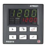
Programmer 72x72mm, single control loop. Allows the programming of 15 cycles/programs that can provide up to 45 steps/segments, all of which can be configured by the user as raise/maintain/lower. Programming mode of the work cycle that is intuitive and simple to use even for inexpert operators.
