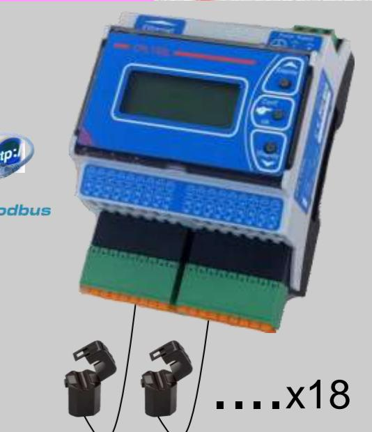
[Communicating sensor for direct current voltmeter and wattmeter in option](#)
